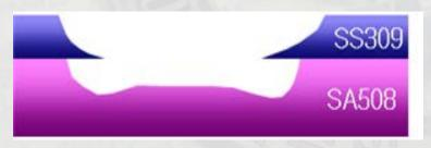
Designed SA 508 thickness = 163.3mm
